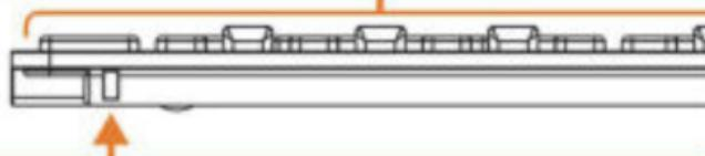
● LED LED flash when the computer is recognizing the device. LED lights on when under normal operation.
