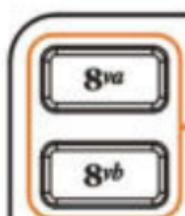
● OCTAVE +/- Press two buttons simultaneously to reset to default. Holding two buttons simultaneously and connect to computer for factory reset.
