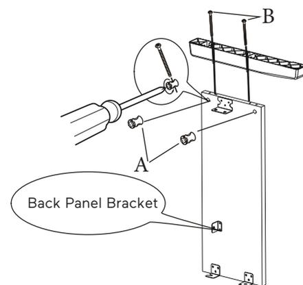
Place the dowells in the feet into the appropriate holes in the bottom of the Stand Legs. Make sure that the feet are facing away from the back panel bracket as shown below. Thread two Foot Bolts (B) through the foot and into the cylindrical washers, rotating the washer to align if needed. Firmly tighten & repeat for the other side.
