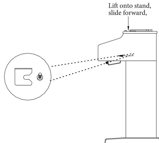
With help from another person, lift the piano onto the stand and slide forwards, pushing the guide rods on the bottom of the piano into the slots on the Stand Legs, as shown below.
