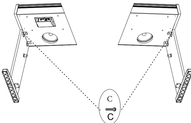
Finish attaching the piano to the stand by using the two Piano Body Bolts (C) to attach the bottom of the piano to its stand.
