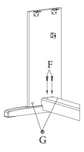
Starting with the right Stand Leg, align the holes in the Pedal Board with the holes in the Pedal Board Bracket as shown. Make sure that the pedals are facing towards the front of the Stand Legs.
