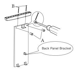
Place the four Cylindrical Nuts (A) into the holes in the Stand Legs, with the screwdriver slot facing out. Use a screwdriver to align the threads in the nuts with the openings on the bottom of the Stand Legs.
