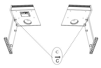
Finish attaching the piano to the stand by using the two Piano Body Bolts (C) to attach the bottom of the piano to its stand.
