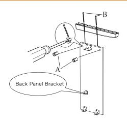
Place the dowells in the feet into the appropiate holes in the bottom of the Stand Legs. Make sure that the feet are facing away from the back panel bracket as shown below. Thread two Foot Bolts (B) through the foot and into the cylindrical washers, rotating the washer to align if needed. Firmly tighten & repeat for the other side.
