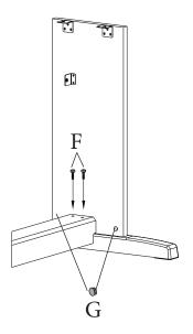
Thread two Pedal Board Bolts (F) through the Pedal Board and into the bracket. Repeat with the left Stand Leg and tighten all bolts fully. Place the four Plastic Caps (G) over the Cylindrical Nut openings.
