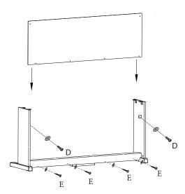
Using two BackPanel Bolts (D) with washers, and four Back Panel Screws (E) with washers, attach the Back Panel to the stand. Please note that the pedal board is not predrilled for the Back Panel screws, and they must be driven in manually.
