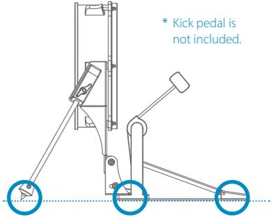
\* Make sure that the three points firmly make contact with the floor using the adjustments below.
