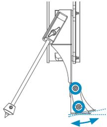
\* Adjust the angle of the base plate if your kick pedal is unstable. (Loosen four bolts to adjust.)
